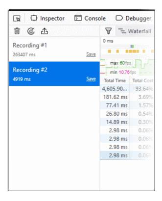
The upper half of the loaded profile displays a time verses call stack size bar-graph of the profile. The call stack represents the amount of active functions at the time when the sample was taken.
